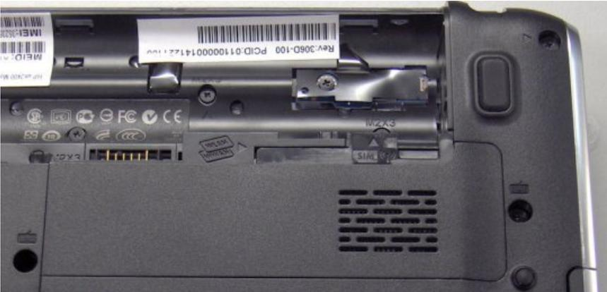
Figure 2: SIM Slot with Cover Removed
